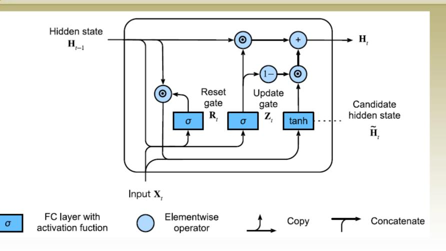
Hidden state computation in a GRU. The multiplication is carried out elementwise
