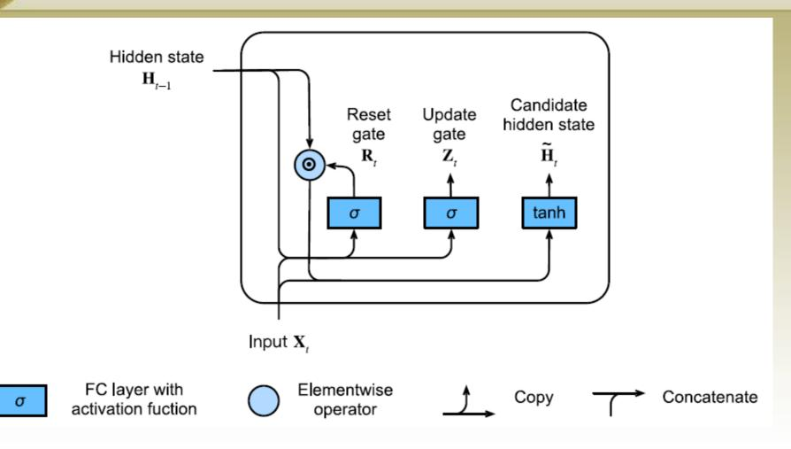
Candidate hidden state computation in a GRU. The multiplication is carried out elementwise.
