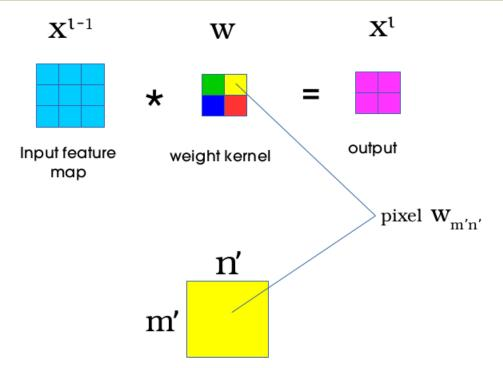
During forward propagation, the convolution operation ensures that the yellow pixel  $w_{m',n'}$  in the weight kernel makes a contribution in all the products (between each element of the weight kernel and the input feature map element it overlaps)
