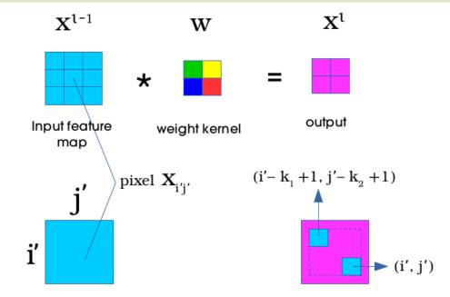
From the previous diagram, we can see that region in the output affected by pixel  $x_{i',j'}$  from the input is the region in the output bounded by the dashed lines where the top left corner pixel is given by  $(i'-k_1+1, j'-k_2+1)$  and the bottom right corner pixel is given by (i',j')
